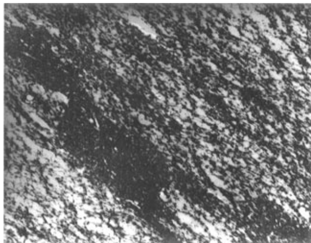
Figure 5. Transmission electron micrograph of an IPN composed of polymers 14 and 17 .
